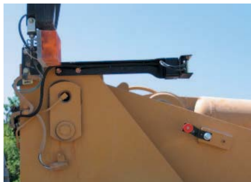
Cat Pox switch installation
